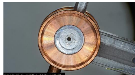
Figure 2: image showing the Cu shield, polypropylene and the CHBr disc from one side. On the right is the the backlighter. The 3D pinhole tube defines the xray backlighter distance. The Cu tube from the bottom is used to fill the chamber with gas to a pressure of 1bar. Figure 3 above shows the backlighter target.
