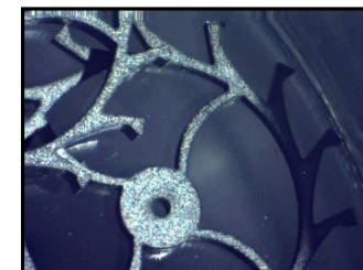
200 \mu m thick tungsten 200 \mu m arm width Inner circle: ID 170 \mu m OD 1.3mm
