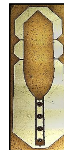
laser profiling: 25 \mu m thick polyimide 4.2mm length 840 \mu m width 150 \mu m diameter holder with 75 \mu m excimer drilled wells
