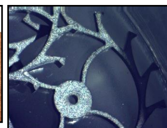
200µm thick tungsten 200µm arm width Inner circle: ID 170 µm OD 1.3mm
