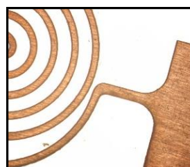
200µm thick copper 100µm arm width
