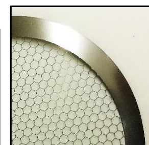
50µm thick niobium 50µm arm width
